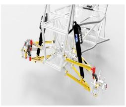
Fig. 6. Double Wishbone suspension system
